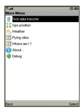
Make sure you went through the "Connect your Bluetooth GPS" section. When the GPS is locked on the satellites, select "Gps position" and your latitude/longitude/altitude should be available.
