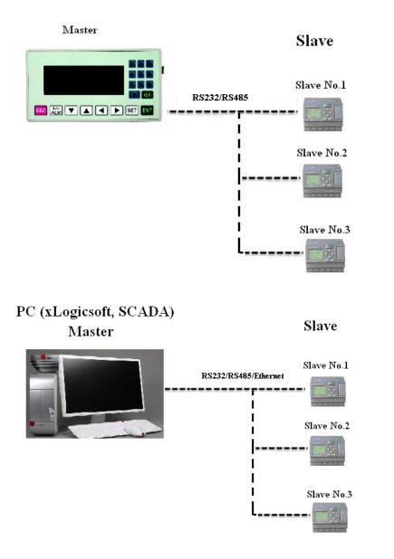
At present xLogic supports baud rate: 9600. The default is 9600. The default is non parity checking mode. MODBUS RTU is used as communication protocol of xLogic. The defaulted communication protocol is MODBUS RTU format .Defaulted address: 1, and legal address range: 1~247.
