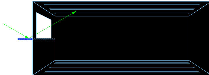
Figure 7.28: Component case study 3: light shelf caustic
